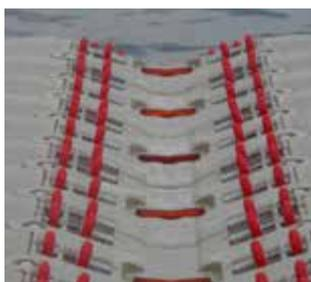
Our Jet Ski drive-on dock is constituted by **several elements**. At first, **modular floating cubes of 50cm x 50cm x 40cm** impart the platform a floating **capacity of 350kg/m<sup>2</sup>**. Next, the **central slipway elements of 1m<sup>2</sup>** equipped with **horizontal and side rolls** gets the hull of the boat.
